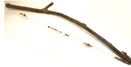
A cotton striking bow (wata-uchi yumi) An instrument for untangling the fibre
