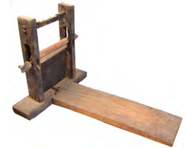
A cotton ginning machine (watakuriki) The seeds are removed by rollers
