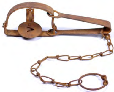
torabasami a heavy steel trap, literally Tiger Shears A hole was dug in the ground, the trap was put in and covered with leaves.
